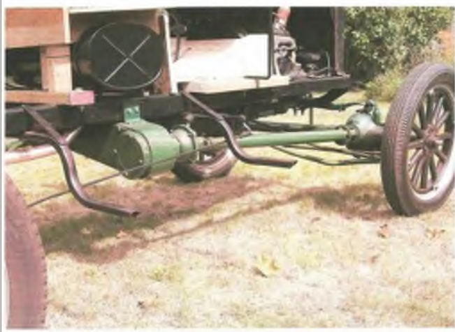
Geoff Reddish of Tasmania sent in the Model T pictures illustrating a four wheel drive modification.
