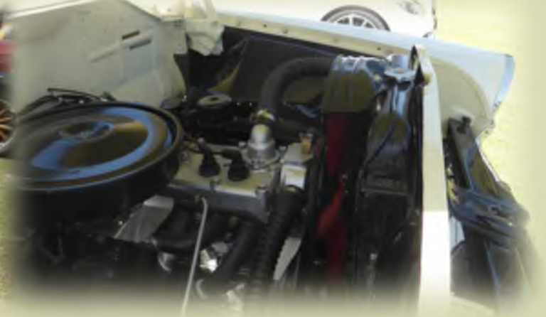
Chrysler Royal's 4.1 litre side valve six cylinder engine
